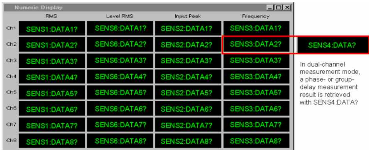
Figure 6-1 Indication of results in the numeric display and associated remote control commands
